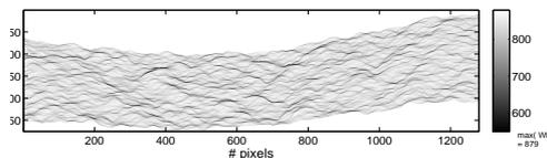
Figure 1. Gray-scale image of the waiting time matrix obtained from 12000 front positions, recorded with a  $1280 \times 276$  pixels resolution at 100 fps. The darker parts correspond to the longer waiting times.
