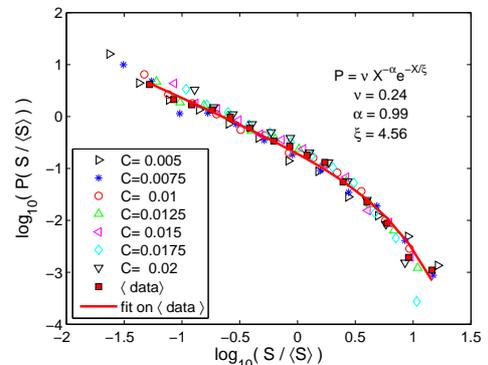
Figure 2. Statistical distributions of avalanche sizes for a given set of experimental parameters. The different distributions are obtained by keeping the velocities larger than a given threshold  $v_c$ , defined by  $v_c = \langle v \rangle + C(\max(v) - \langle v \rangle)$ , where  $C$  is the clip level.
