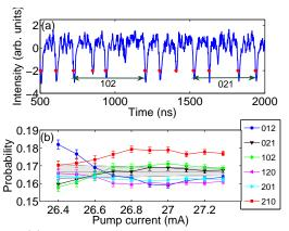
FIG. 1. (a) Experimental time trace of the laser intensity. The red dots indicate the spike times and two ordinal patterns (words) are indicated as examples. (b) Probabilities of the different patterns versus pump current.
