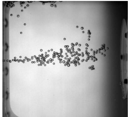
Figure 1. Jet of bubbles in a cubic cavity of 10 cm side in microgravity conditions 1 from a drop tower experiment.
