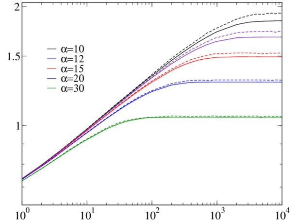
FIG. 2. Width of a droplet as a function of time for a given contact angle. Dashed lines represent stochastic films while continuous lines represent deterministic films.
